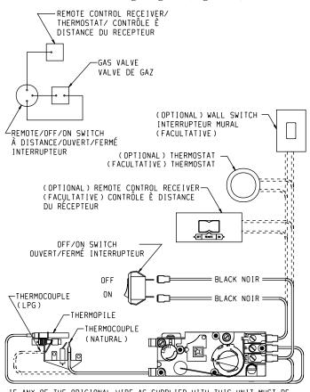
IF ANY OF THE ORIGIONAL WIRE AS SUPPLIED WITH THIS UNIT MUST BE REPLACED. IT MUST BE REPLACED WITH NO. 18. 150°C WIRE OR ITS EQUIVALENT.
